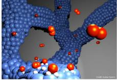
Illustration of a network of nano-wires: The high surface area is achieved by the platinum–cobalt bone nanostructure and the nano-wires are conducting themselves so the carbon material is not needed for electronic contact.
