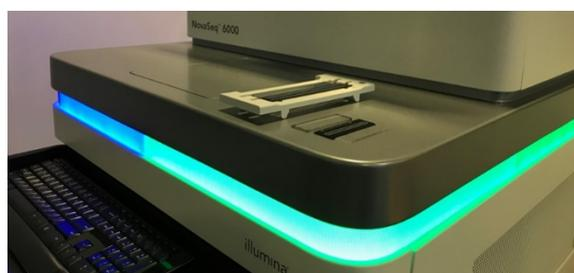
**The Illumina NovaSeq 6000**, which is part of the co-funding from SDU, was purchased ultimo 2017 and installed in January 2018. This new instrument is essential for the work in ATLAS and has greatly improved our sequencing capacity and quality as well as significantly reduced the cost of sequencing. The NovaSeq 6000' data output is at least a 10-fold upgrade compared with the previous Illumina HiSeq 1500 instrument.
