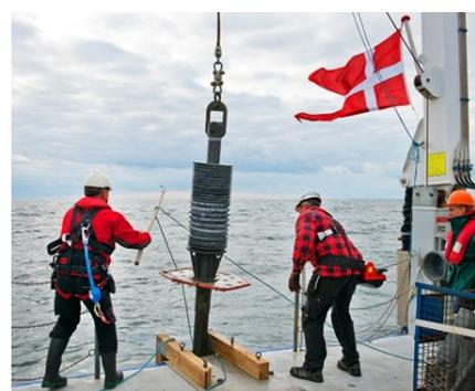
*A gravity core is retrieved from the Baltic seabottom for methane studies on board the research vessel, Aurora.*
